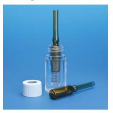
For use in dissolution vessels. Three prongs hold the capsule in place, permitting the completion of dissolution tests without capsule flotation.
