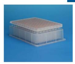
Glass inserts loaded in the 96-well plate performs similar to standard 12x32mm vials for Chromatography testing. 96-well pierceable Cap Mat is lined with the same PTFE/ Silicone septa used in closures for Chromatography.
