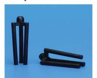
For use in dissolution vessels. Three prongs hold the capsule in place, permitting the completion of dissolution tests without capsule flotation.
