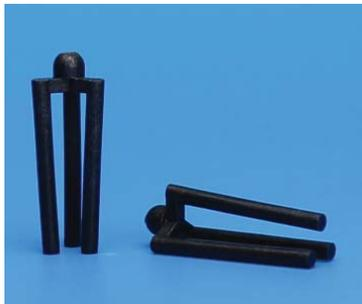
For use in dissolution vessels. Three prongs hold the capsule in place, permitting the completion of dissolution tests without capsule flotation.
