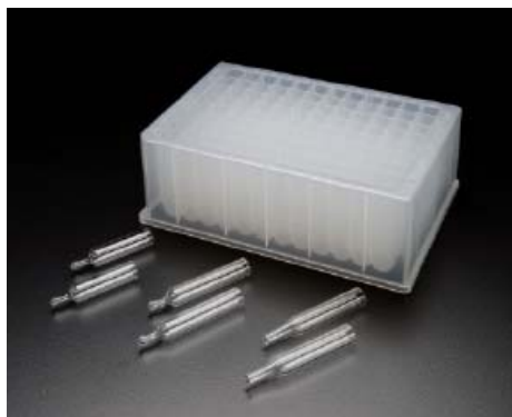
System uses 96 glass tapered inserts in a 96-square deep well plate.
